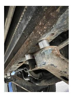
With previous shock removed, Swaybar unbolted from the links and mounting point, insert the two relocation plates to sway bar mounting point with reservoir bracket in between. Once relocation plate is in position remount sway bar to plate.
