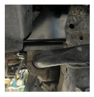
Once this is complete, the shock can be inserted into the tower and bolted in. Make sure that the hose from the top of the shock is pointing to the front of the vehcile for reservoir positioning. Ensure that the lower shock mount has the rebound adjuster pointing inwards.
