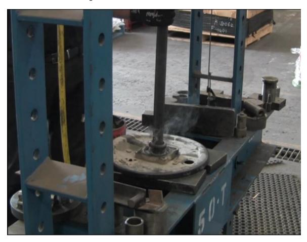
Remove the retaining collar and spacer, please note how the spacer was fitted.
