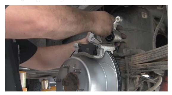
Remove clamps from flexible brake hose.
