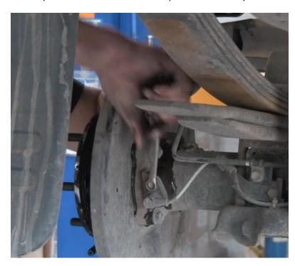
Remove the handbrake retaining clip and cable.
