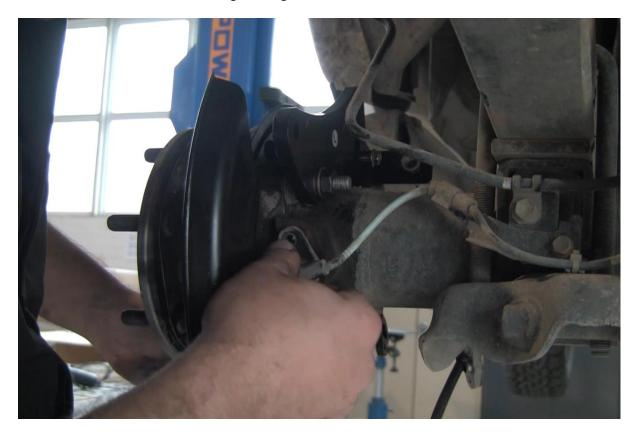
Refit handbrake assembly and hand brake cable onto the backing plate. #9 & #22  $\,$
