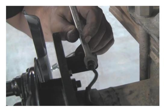
Before fitting the new brake rotor, make sure the axle face is clean.
