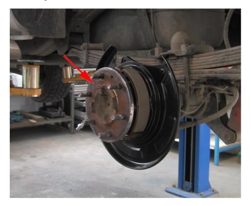
Fit the new brake rotor.
