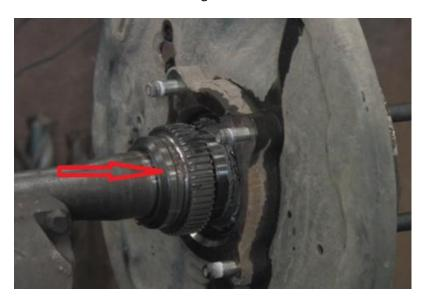
Knock out the four studs from the axle bearing housing.
