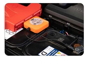
The Ultimate9 BM app is simple to use, and not only monitors battery voltage, but will run cranking and charge tests as well as including a trip function to monitor charging periods while you drive.
