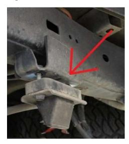
1.Remove the rubber bump stop on the chassis. Using the original bump stop bolts secure the top bracket to chassis.
