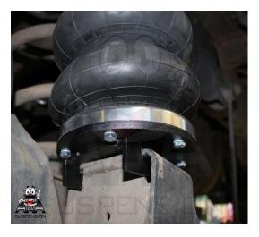
3. The L piece bolts to the other side of the lower bracket to prevent it from moving forwards and the claws from escaping their grab on the strike plate.
