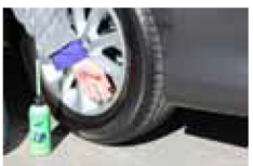
3. Remove top from bottle as it contains a built in valve removing tool. Remove rubber valve cap from tyre.
