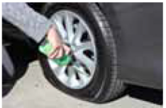
5. Once the tyre is fully deflated, place filler tube over valve opening and squeeze contents into tyre.
