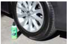
7. Re-inflate tyre to recommended pressure and rotate several times to evenly spread contents.
