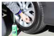
4. Simply fit valve remover over exposed valve core then turn anti clockwise until tyre begins to deflate.
