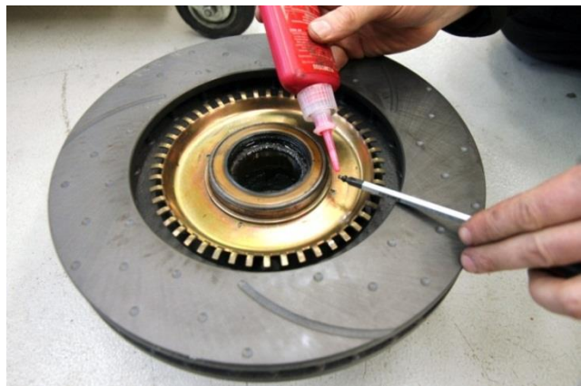
Image 2.2 Tightening the screws holding the reluctor ring
