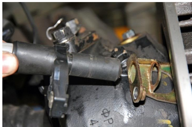
Image 4.1 Removal of the O-ring prior to inserting into bracket.
