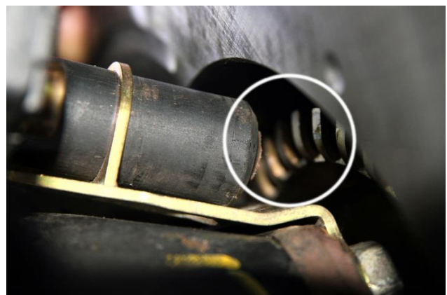
Image 4.3 Clearance (exaggerated) between ABS sensor and reluctor ring.
