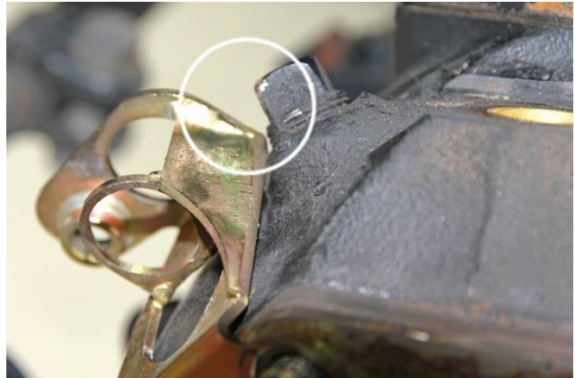
Image 3.3 Clearance beside the ABS sensor mount.
