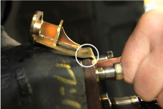
Image 3.2 Clearance under the ABS sensor mount
