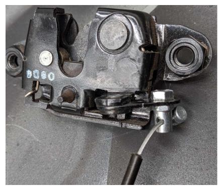
7. Refit the black sheath over the wire then pass the other end through the white clip that the corresponding release rod was connected to in the centre of the tailgate and fit another wire clamp on the opposing side. Do not tighten this clamp or trim the wire yet, you will adjust this properly after the storage box has been installed. If you tension the wire now the storage box will not be able to sit into the tailgate correctly. Repeat the cable conversion with the latch on the other side
