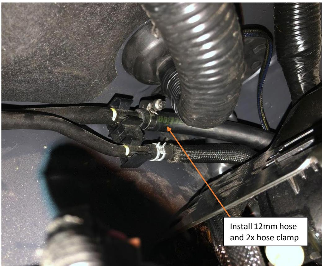
8. Route the 12mm fuel hose around the factory filter and down the inner guard to the Inlet port of the Ryco filter.
