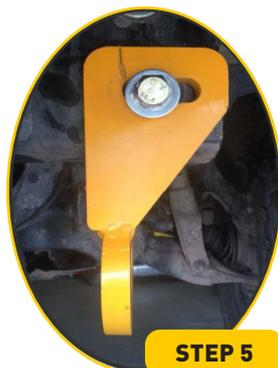
1. Place tow point into position by sliding over front bumper assembly.
