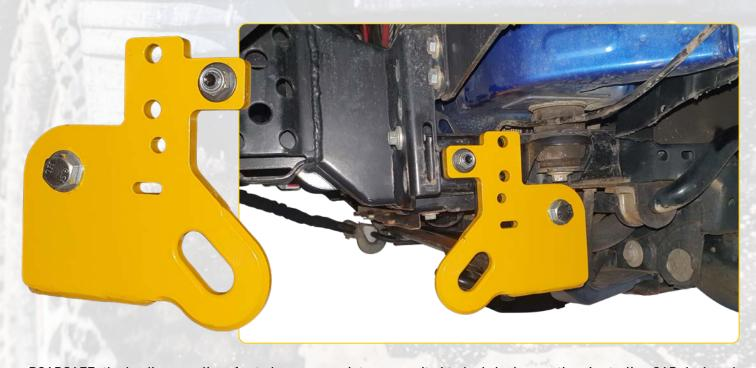
ROADSAFE, the leading supplier of rated recovery points, are excited to be bringing another Australian CAD designed, engineered & RATED recovery point product to the market. Now featuring an internal radius teamed with an external chamfer around the shackle eye, for improved soft shackle compatibility to prolong longevity of the ROADSAFE soft shackles in recovery scenarios.
