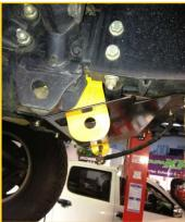
Ensure all supplied and specified components are used during the installation of tow points. Failure to do so will significantly reduce the Working Load Limit (WLL) specified for each individual point, which can result in serious injury or death.
