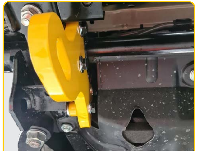
Figure 4 - Undertray in place after notching
