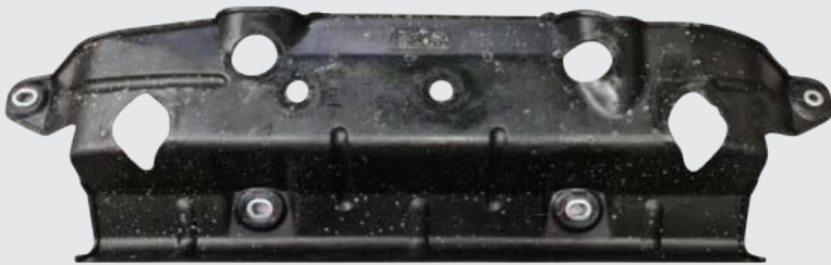
Figure 3 - Notching of plastic undertray
