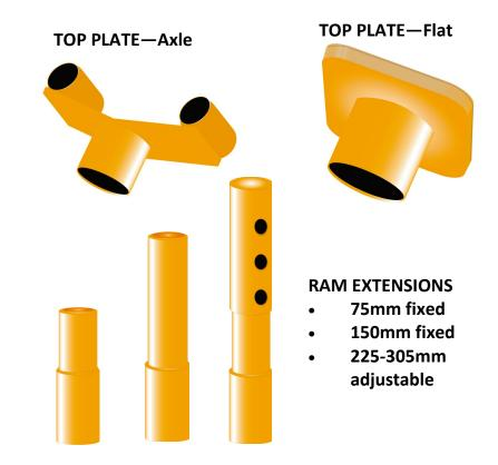
Ram Extensions & Top Plates have been designed standard with 35.5mm ID to suit for a 28-35mm ram OD. Adaptors available to suit for 35.5-39.5mm, 40-44.5mm & 45-49.5mm size rams.
