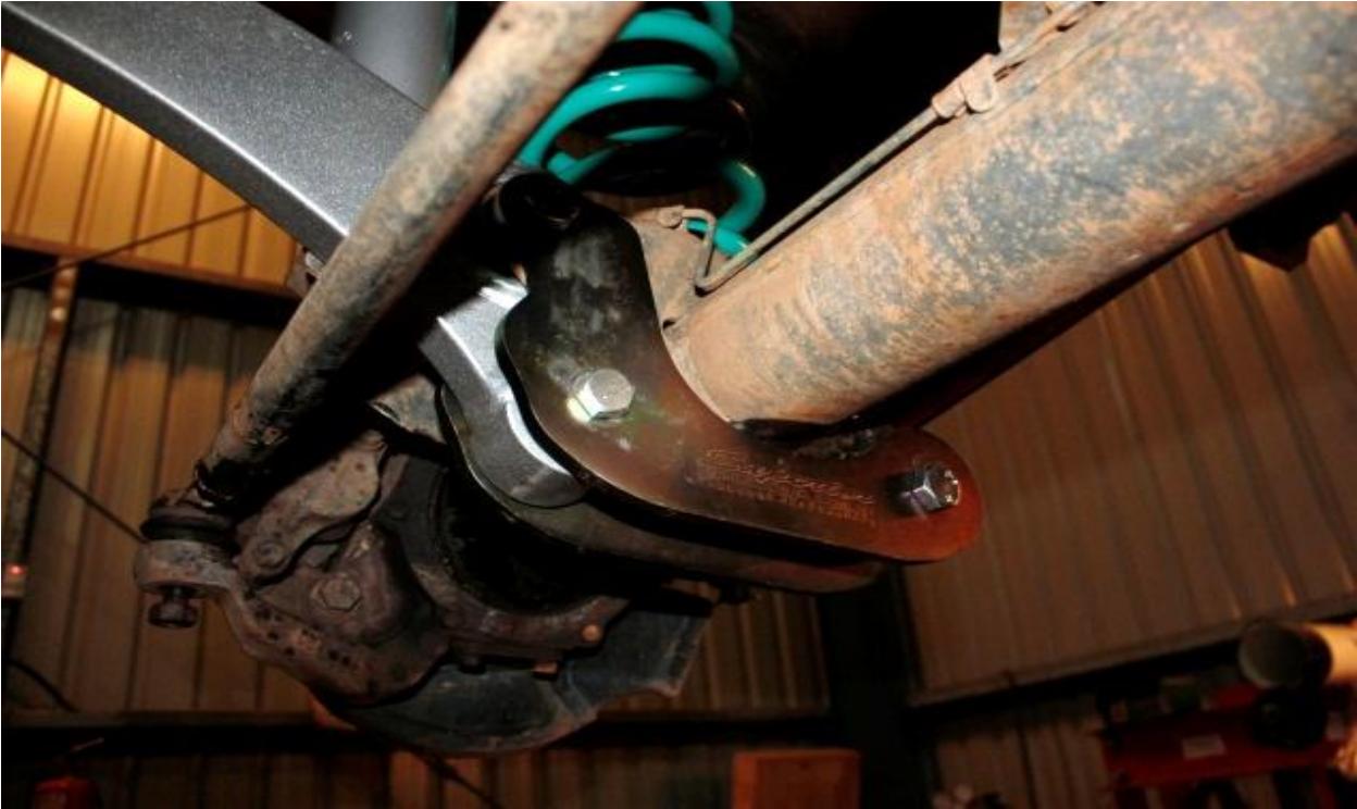
FIGURE 3: SHOWS PLATES FITTED ON THE PASSENGER SIDE
