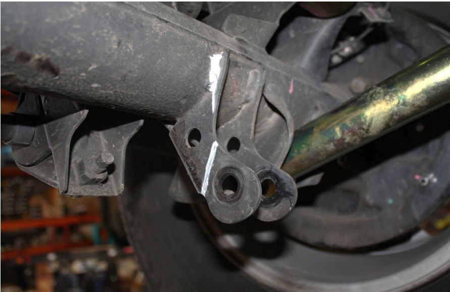
FIGURE 1: CORRECT MARKING OF THE FACTORY SHOCK MOUNT
