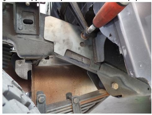
Figure 2: Correct Location Of Chassis Brace Item #1 & #2 - Drivers Side
