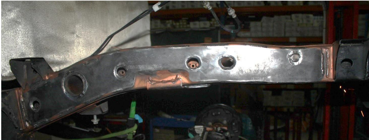
Figure 4: Brace welded in position and cleaned - Passenger Side
