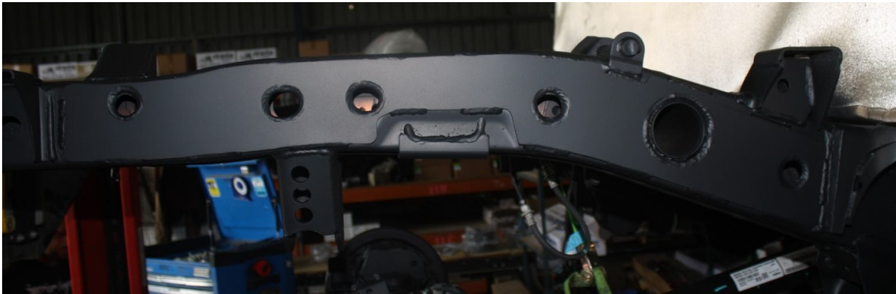
Figure 7: Brace with rust prevention re-applied and painted - Drivers Side
