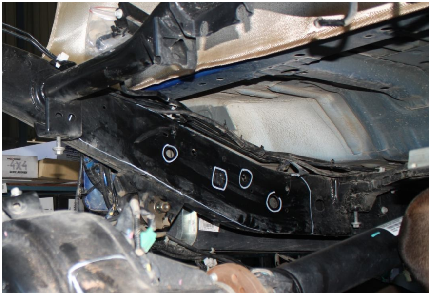
Figure 6: Inner chassis Plate location and preparation prior to welding
