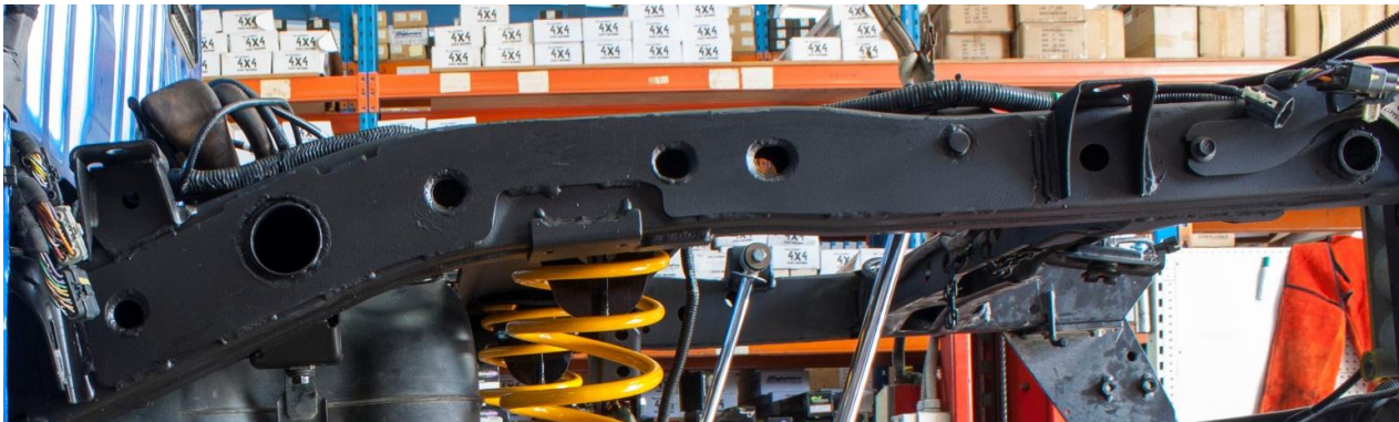
Figure 8: Brace with rust prevention re-applied and painted - Passenger Side
