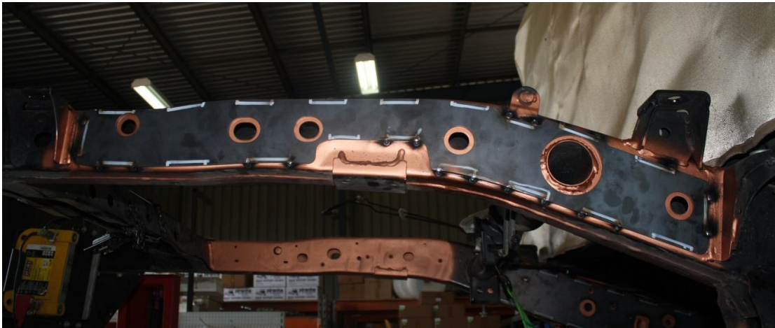
Figure 3: Correct Location Of Chassis Brace Item #2 - Passenger Side
