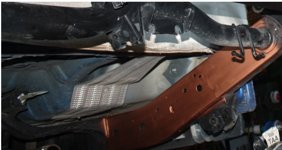
Figure 6: Inner chassis Plate location and preparation prior to welding
