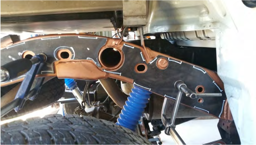
Figure 4A: Correct Location of Chassis Brace Driver Side
