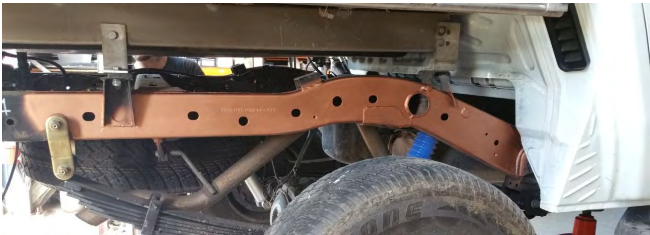
Figure 3: Chassis preparation prior to welding - Driver Side
