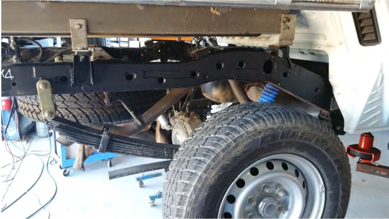
Figure 7: Cleaned, Rust-proofed and painted - Chassis Brace Drivers Side
