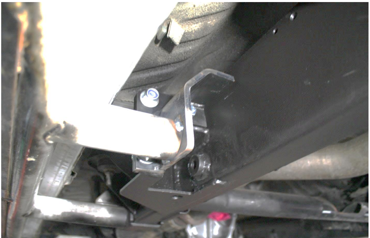
Figure 4: Correctly Fitted Long Arm Slider Mount Rear Shot.
