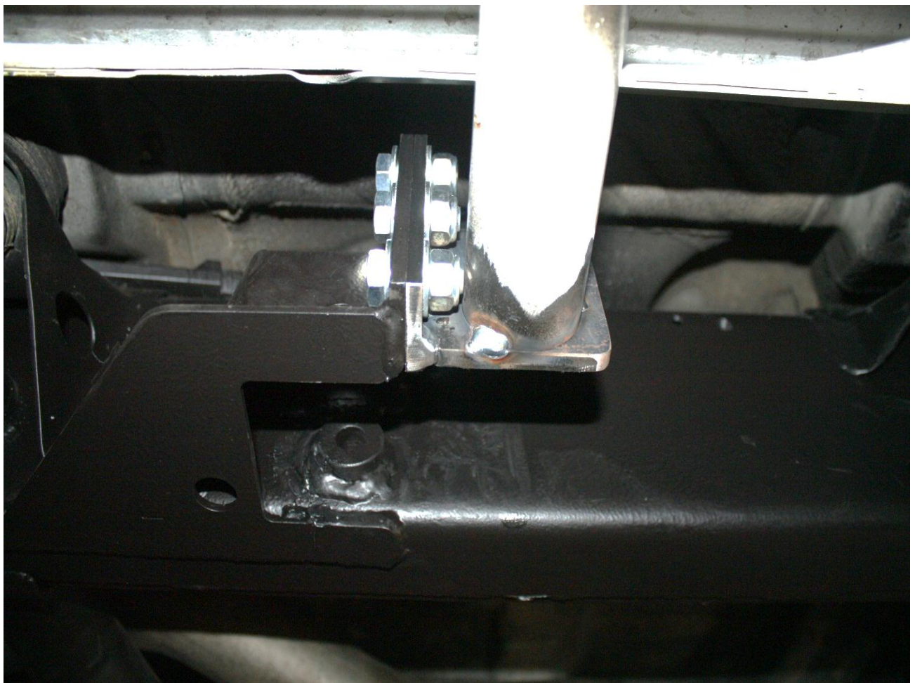
Figure 2: Correctly Fitted Long Arm Slider Mount.
