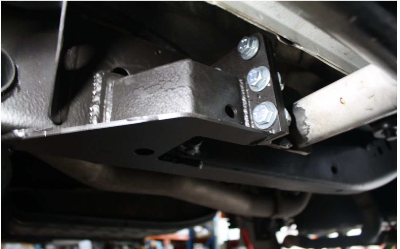
Figure 3: Correctly Fitted Long Arm Slider Mount Front Shot.
