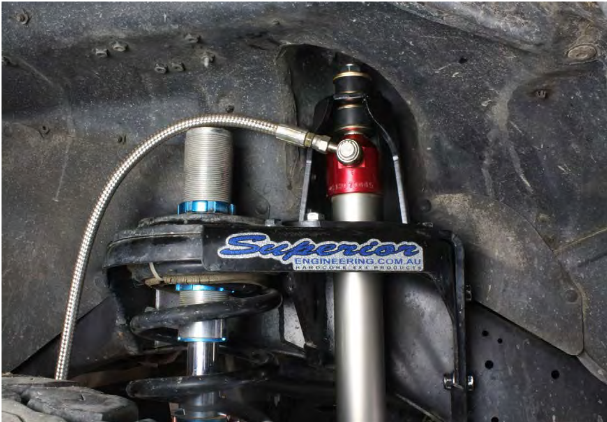
Figure 4: Shock Tower With Shock Fitted With Out remote Reservoir Mounted
