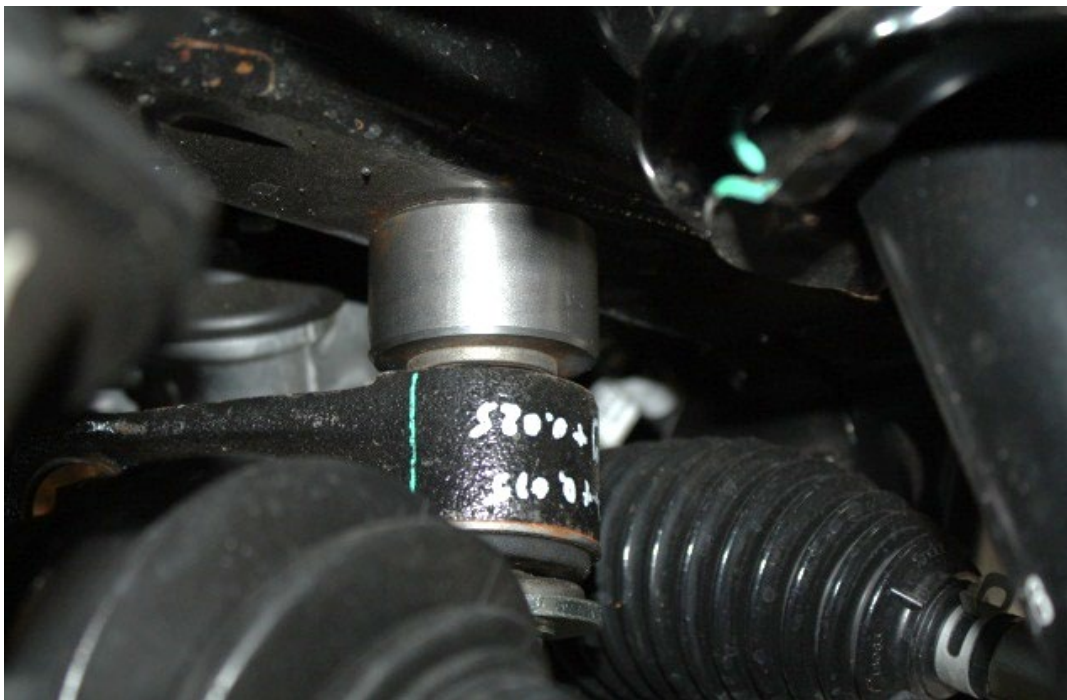
FIGURE 2: CORRECTLY FITTED DIFF DROP BOSS
