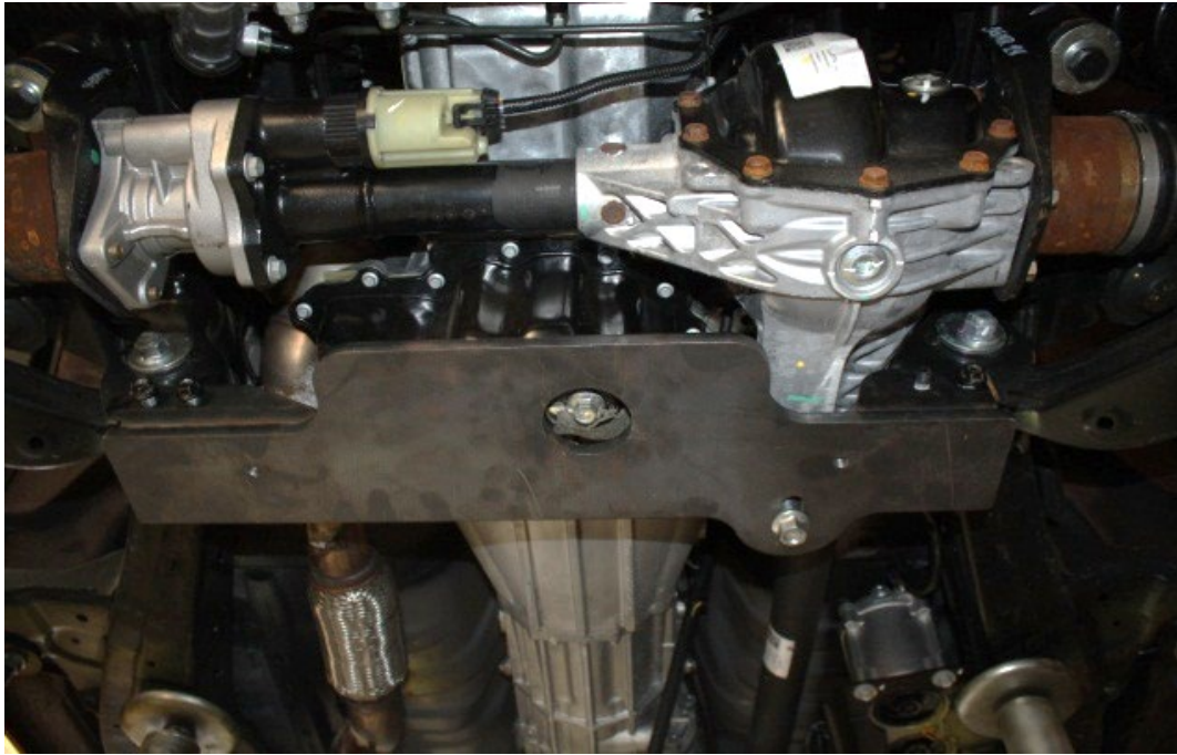
FIGURE 1: CORRECTLY FITTED DIFF DROP CROSSMEMBER
