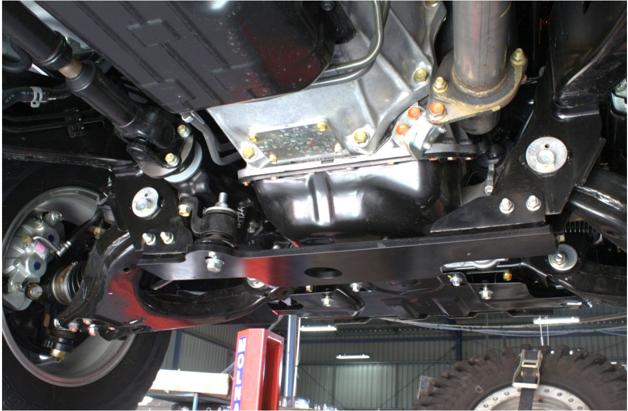
FIGURE 3: CORRECTLY FITTED DIFF DROP
