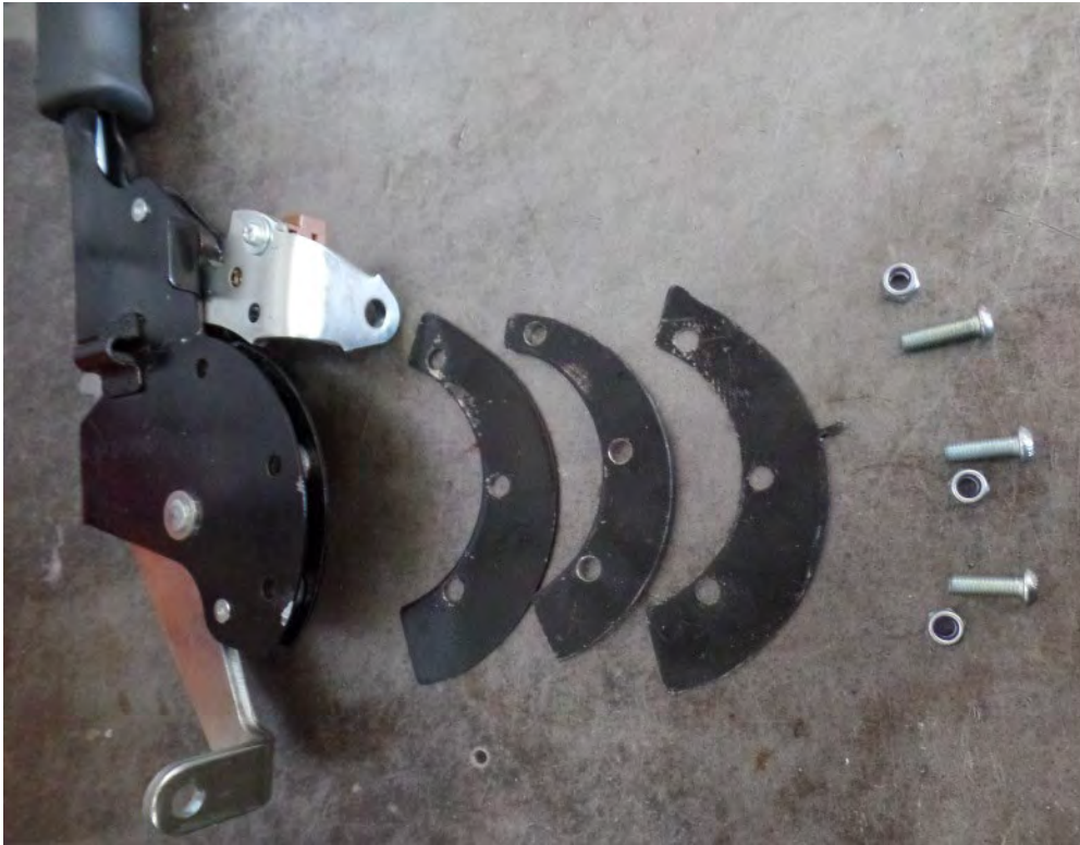
Figure 5: Mount cam plates into position
