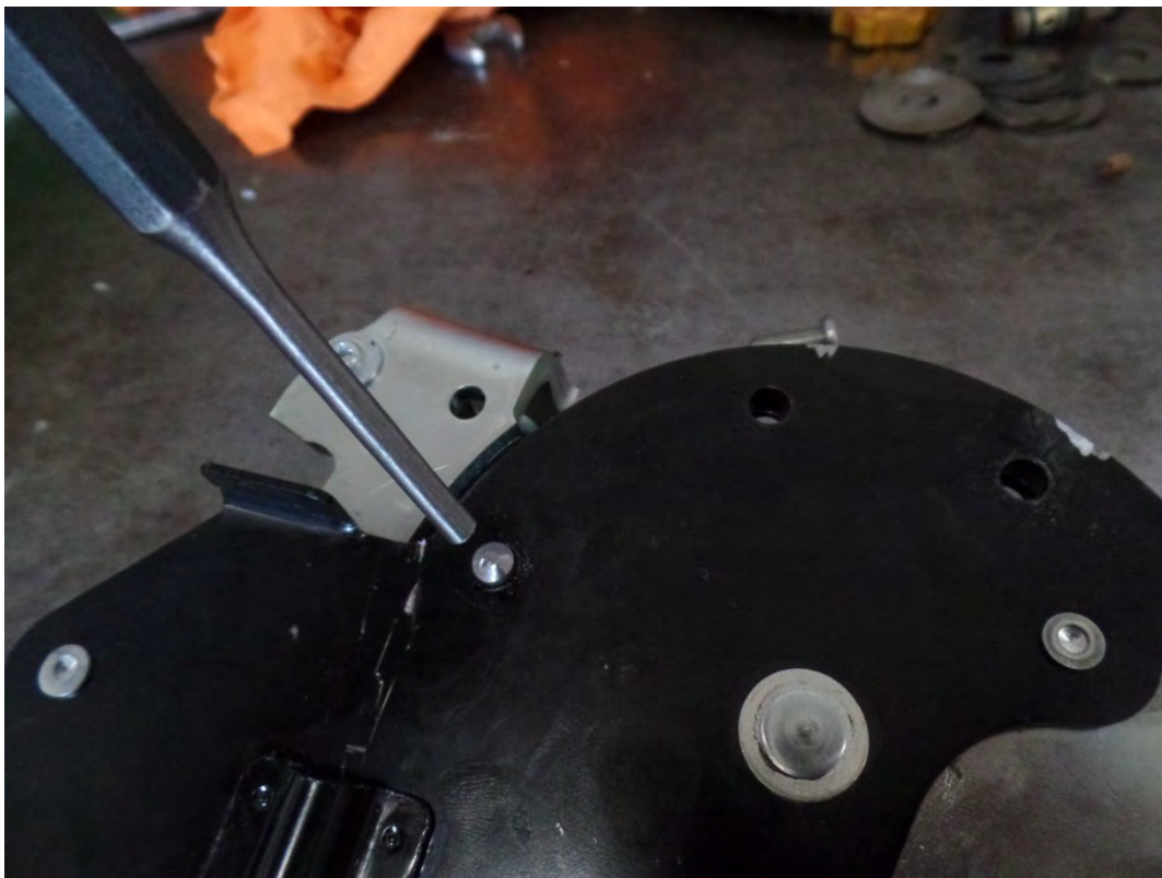
Figure 4: Use pin punch to remove studs (3)
