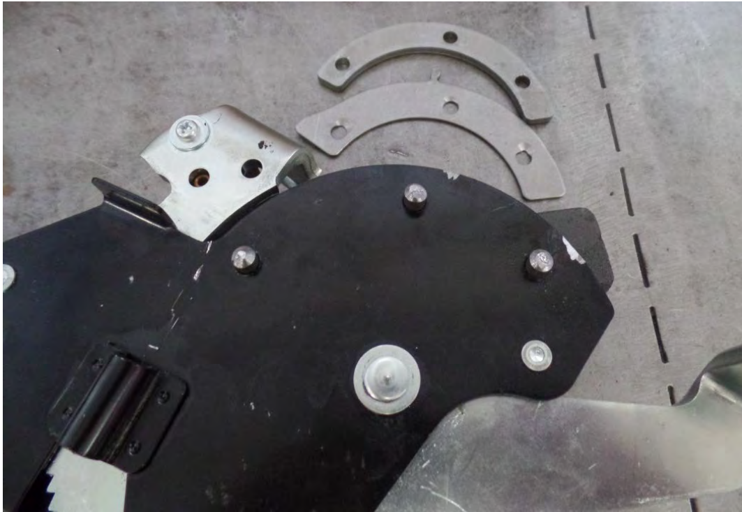
Figure 3: Grind or file studs to allow plate removal
