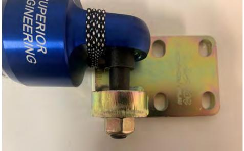
Step 2. Remove the Allen head top bolt (shown with arrow below) and apply permanent Loctite and refit and tighten up to correct torque settings.
