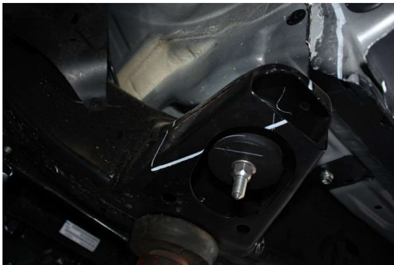
FIGURE 1: CORRECTLY MARKED OUT FRONT BODY MOUNT
