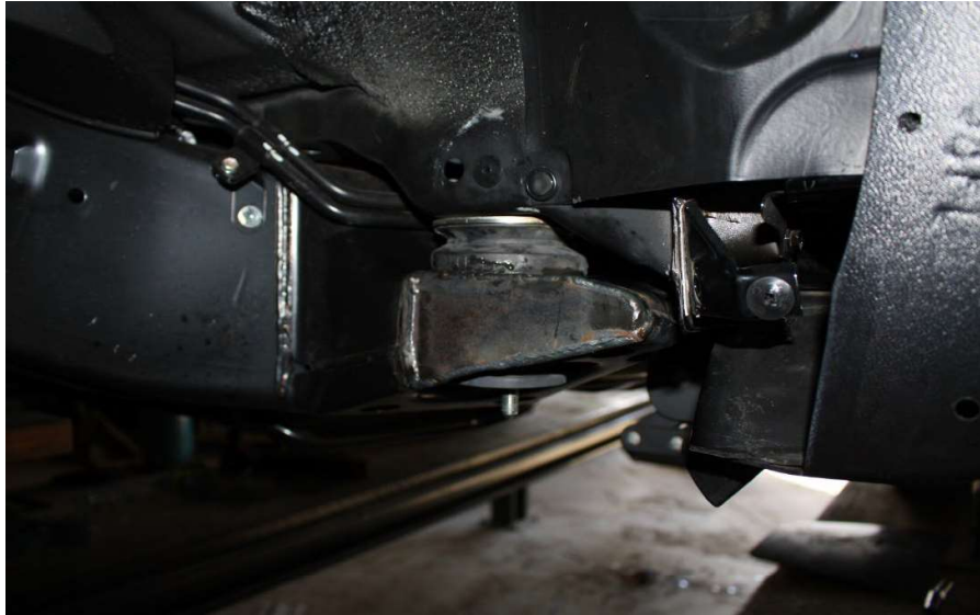
FIGURE 2: CORRECTLY FITTED BODY MOUNT INFILL PLATE
