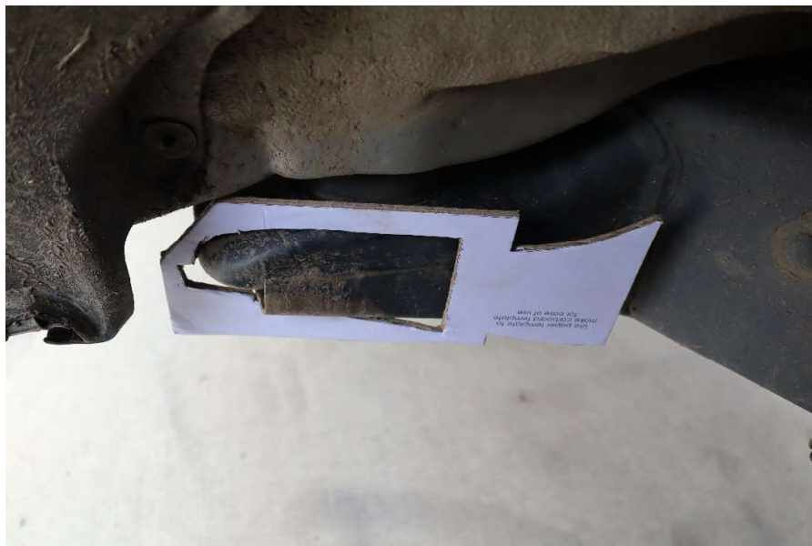
FIGURE 2: CORRECTLY FITTED BODY MOUNT INFILL PLATE
