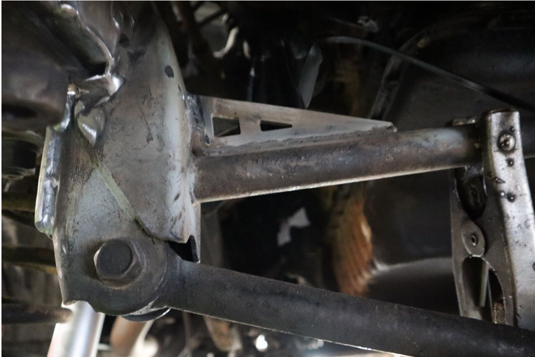
FIGURE 10: Location and placement of large Inner gusset.
