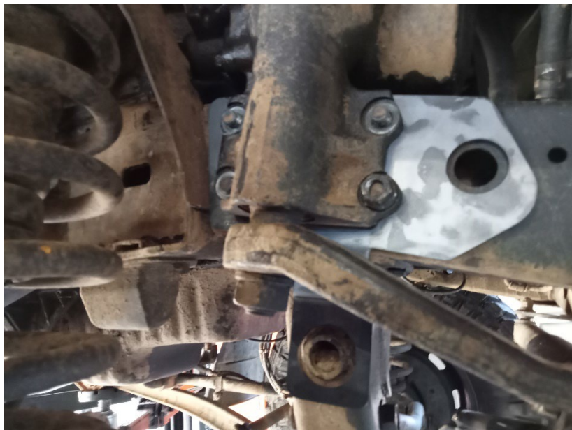
FIGURE 3: Location and placement of Outer Plate
