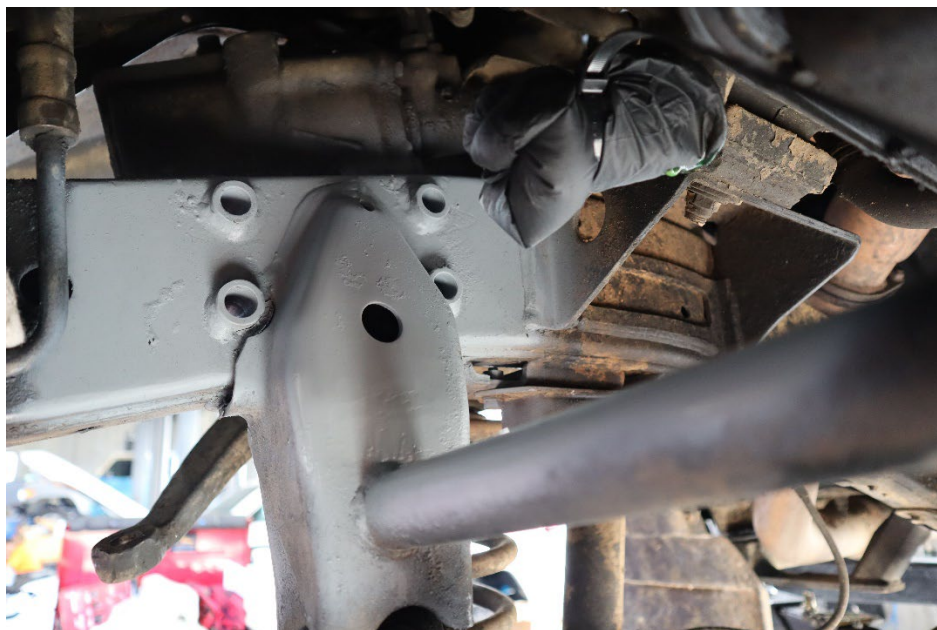
FIGURE 8 & 9: Cleaned area prepped with weld through primer.
