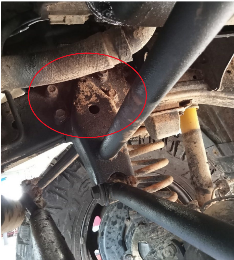
FIGURE 1: Inner Side of Chassis, Bolts to be removed to allow power steering box to move.
