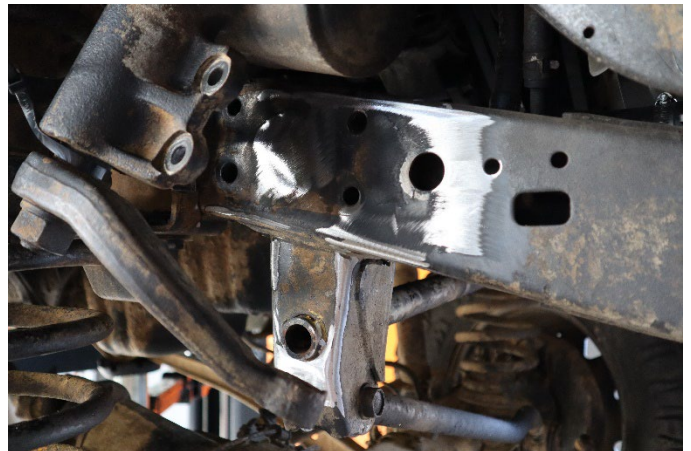
FIGURE 6 & 7: Trace around plate to mark area to remove paint and clean.
