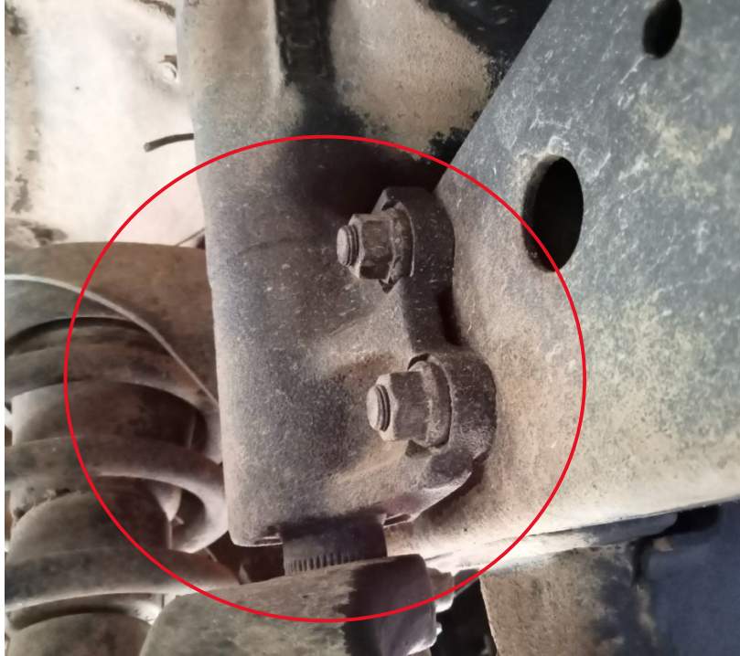
FIGURE 2: Outer Side of Chassis, Bolts to be removed to allow power steering box to move.
