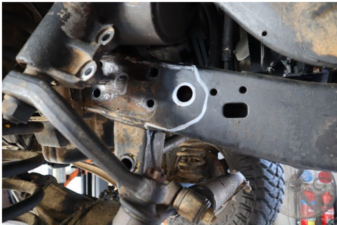
FIGURE 6 & 7: Trace around plate to mark area to remove paint and clean.
