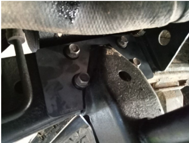
Figure 4 & 5: Location and placement of Inner plate, Trace around plate to mark area to remove paint and clean.
