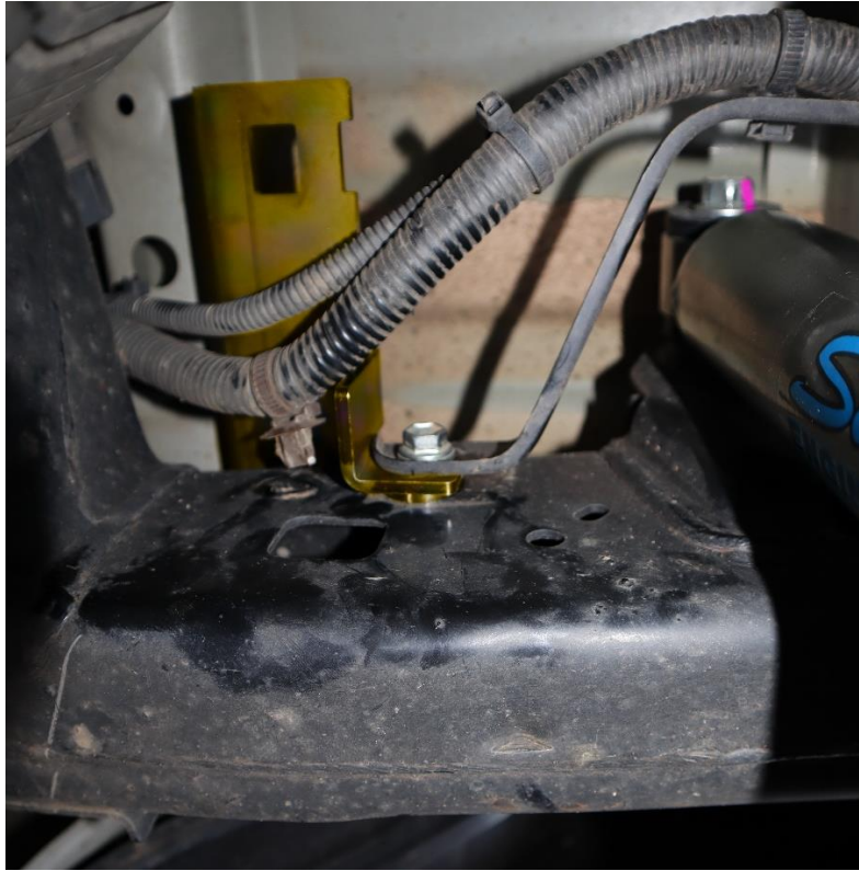
FIGURE 7: Passenger Side – Example of inside of mount showing Washer installed for Vehicles not fitted with Superior Engineering Chassis Brace kit.
