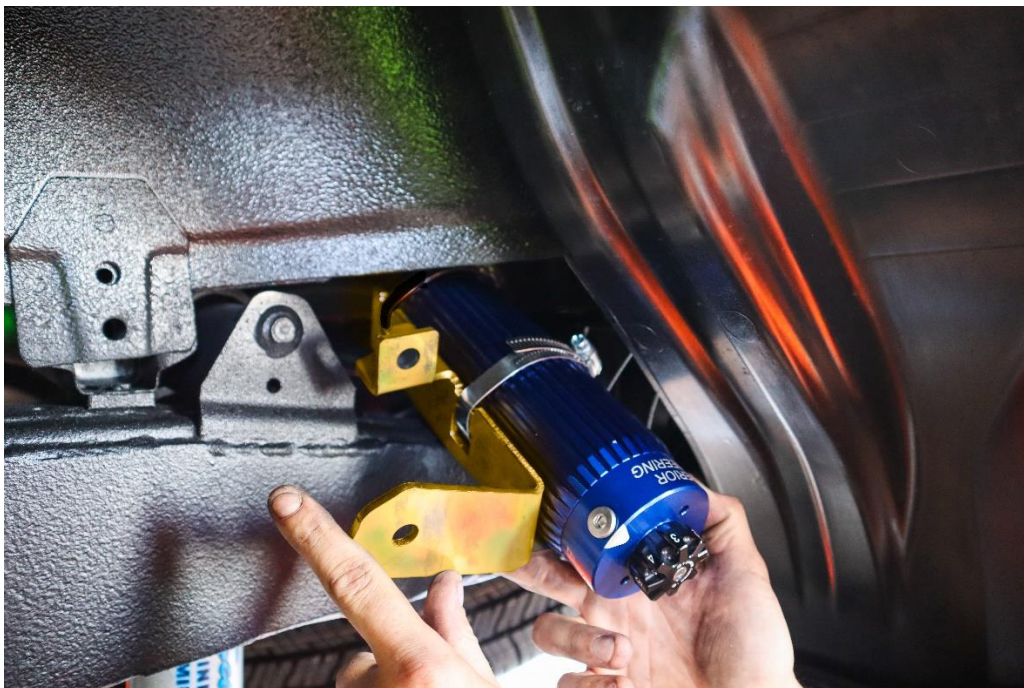
FIGURE 6: Passenger Side – Feeding the mount with Reservoir installed into place.
