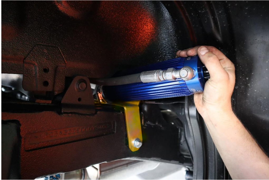
FIGURE 5: Drivers Side - Feeding the Reservoir into the mount, with the adjustment dial on the outside.
