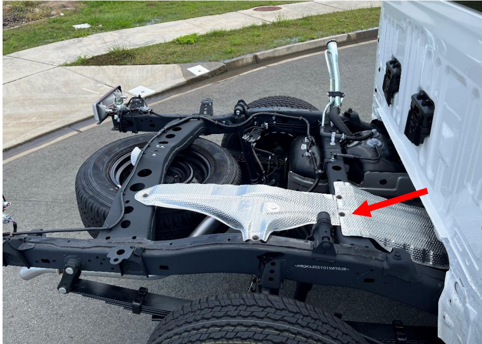
FIGURE 1: Drivers Side - M8 bolt to remove on crossmember.
