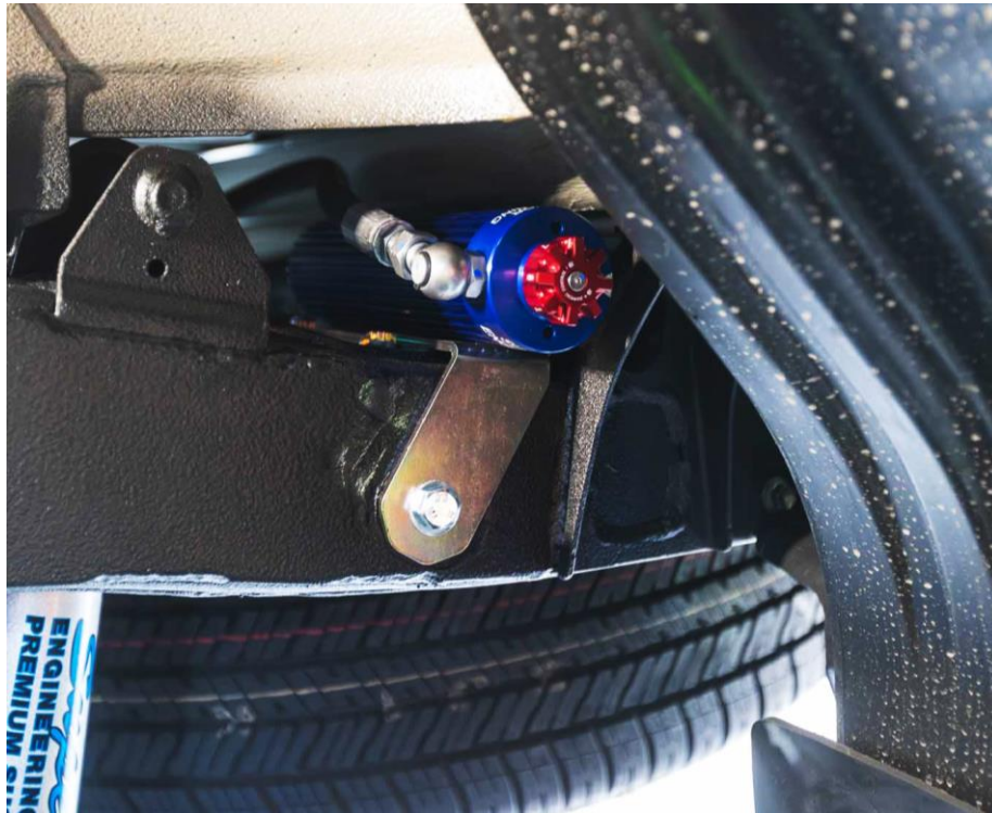
FIGURE 9: Passenger Side – Complete fitted Remote Res mount.
