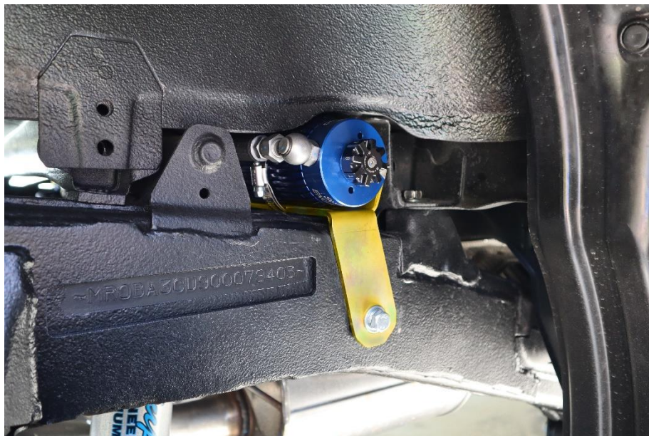
FIGURE 8: Drivers Side – Complete fitted Remote Res mount.
