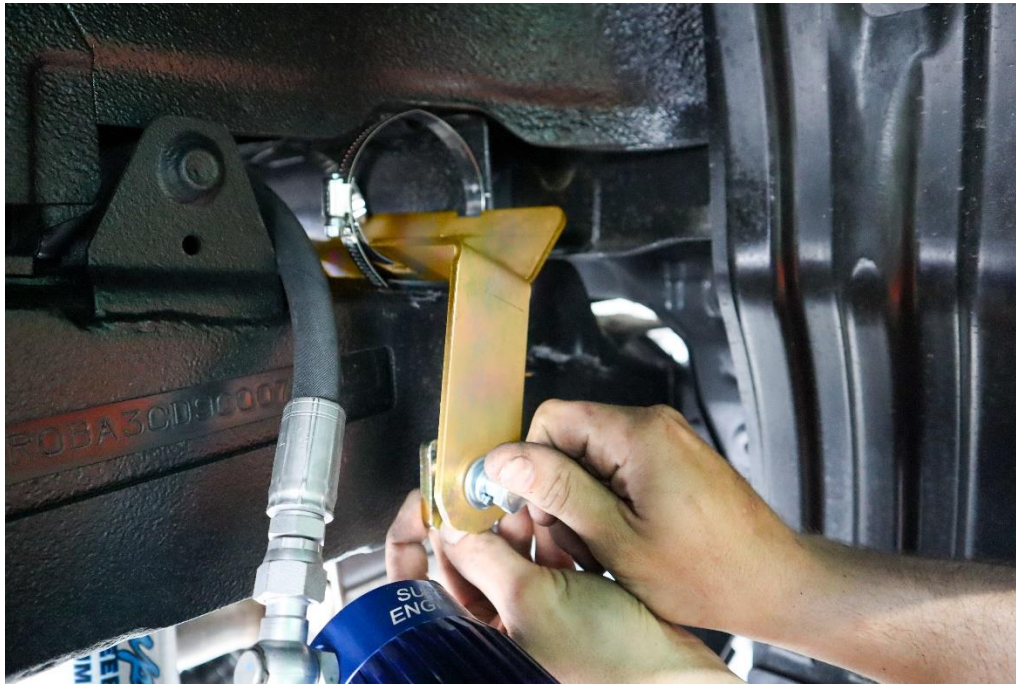
FIGURE 3: Drivers Side - Fitting the Threaded plate and Hose Clamp positions to suit 2.5 Res Shock
