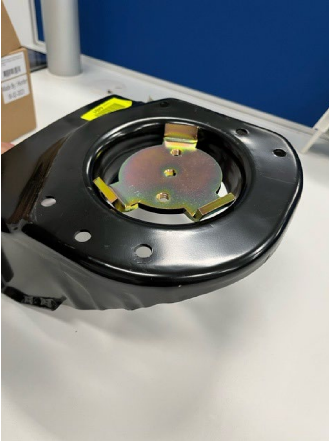
Shows top plate fitted in position
