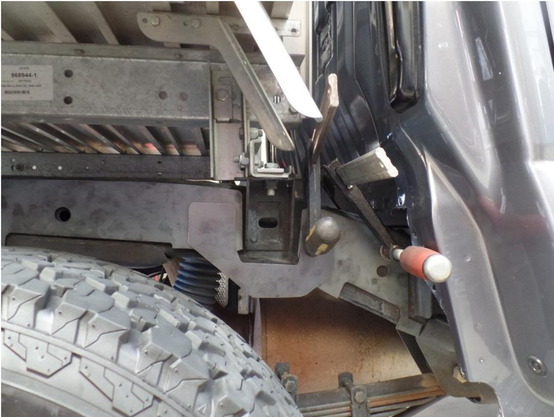
**Figure 3: Correctly Fitted Chassis Brace Item #3 - Driver Side**
