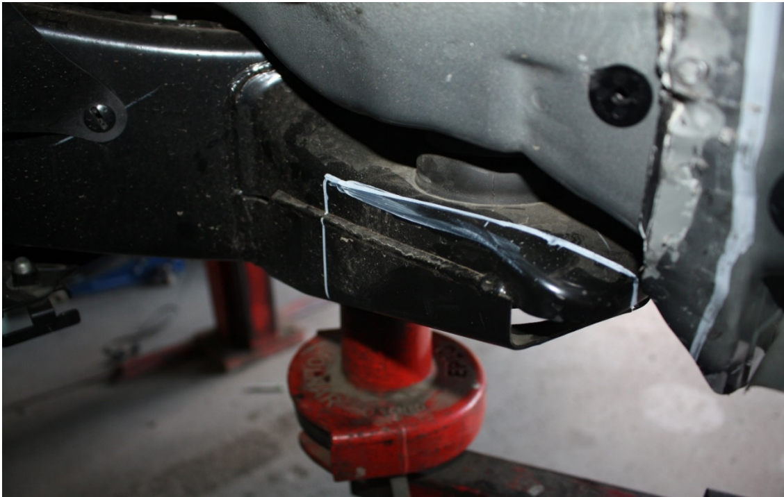
FIGURE 1: CORRECTLY MARKED OUT FRONT BODY MOUNT
