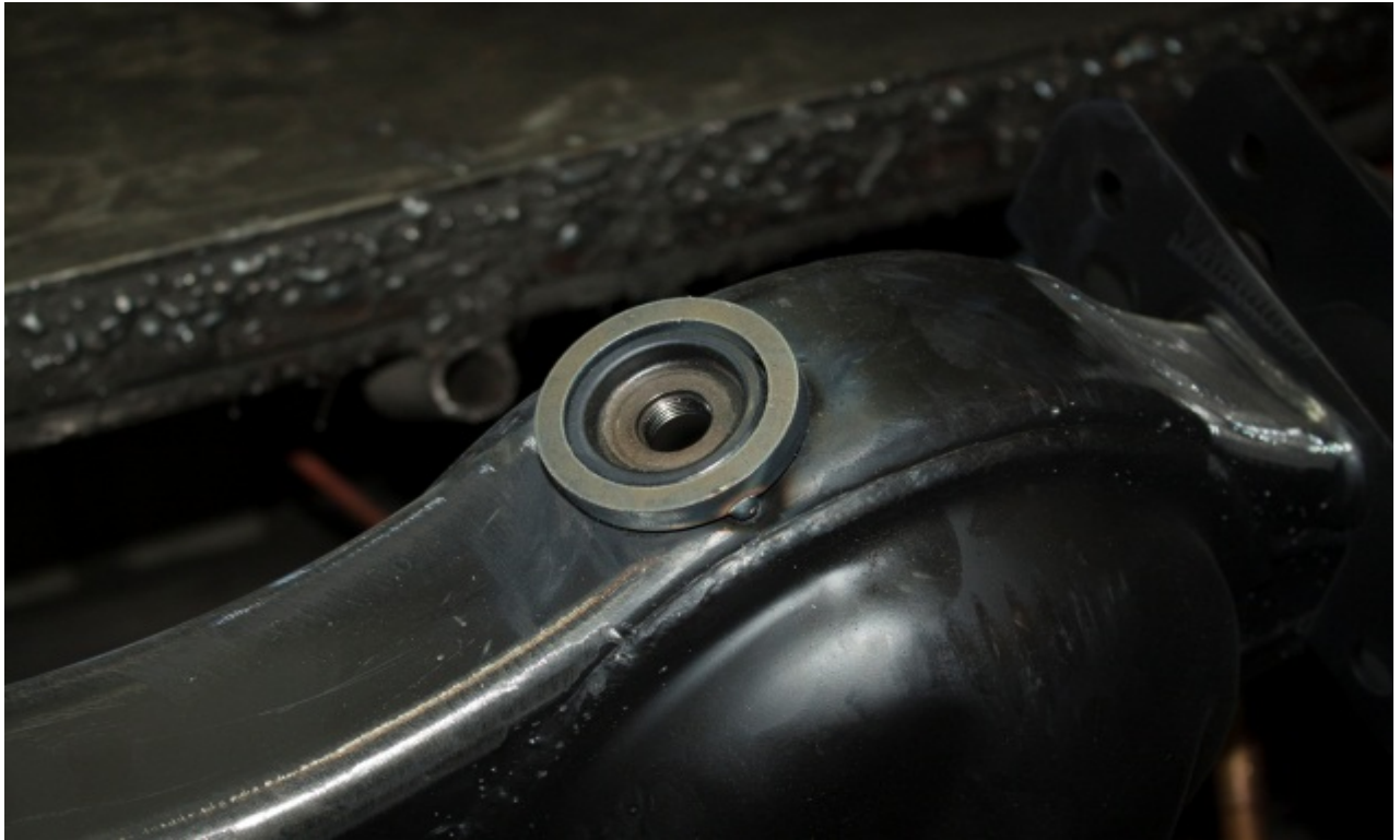
Figure 5: Diff Ring Protector Correct Location
