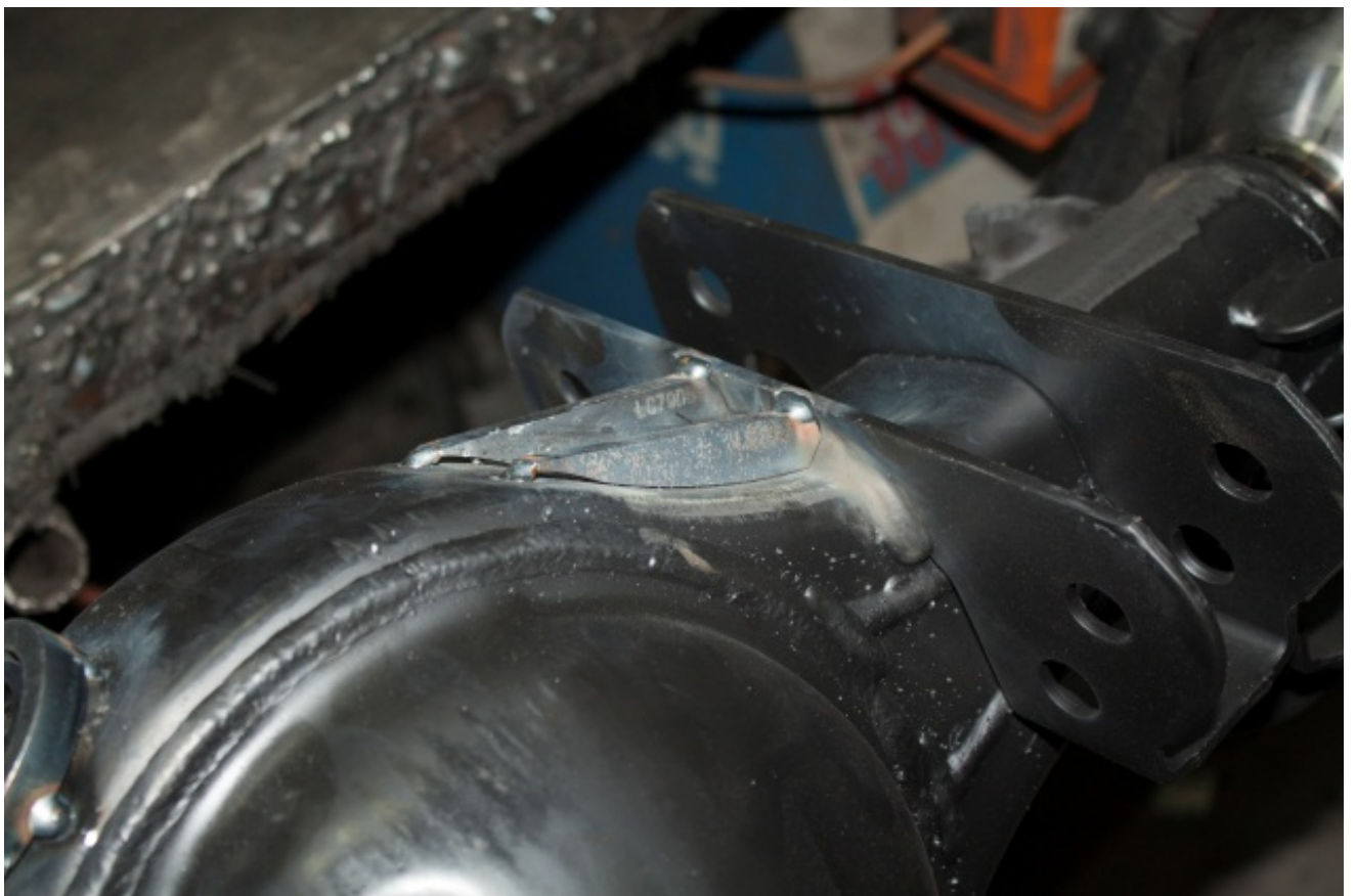
Figure 4: Small Front And Large Rear Gusset Correct Location.
