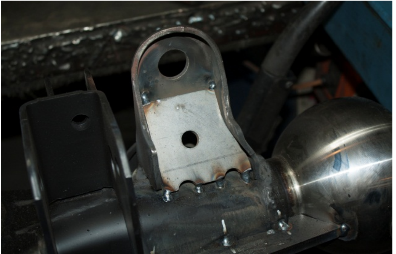
Figure 3: Shock Mount Gussets Tack Welded In Place
