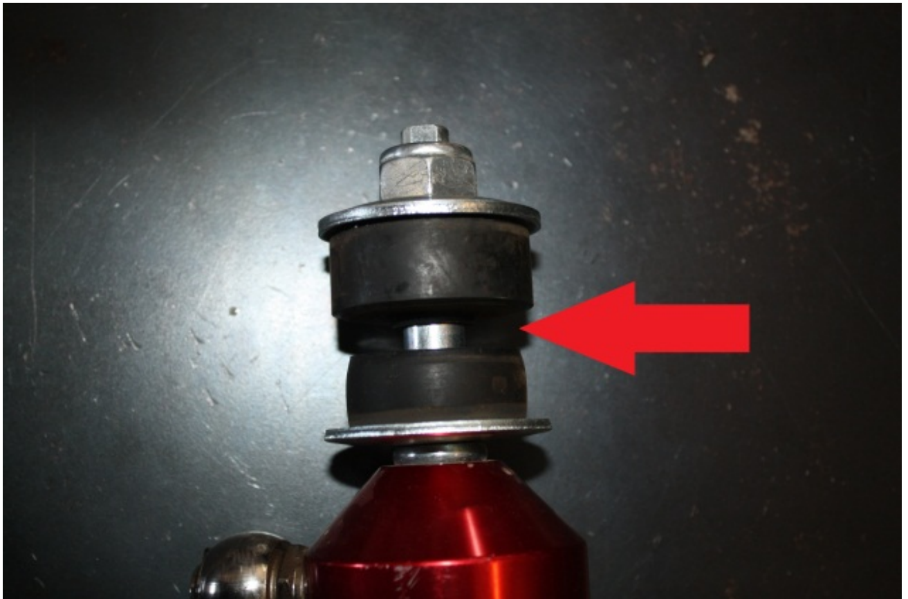
Figure 1: Correctly Fitted Bush Assembly
