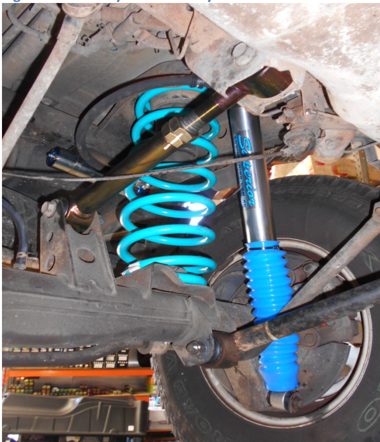
Figure 3: Correctly Fitted Pin Eye Style Shock
