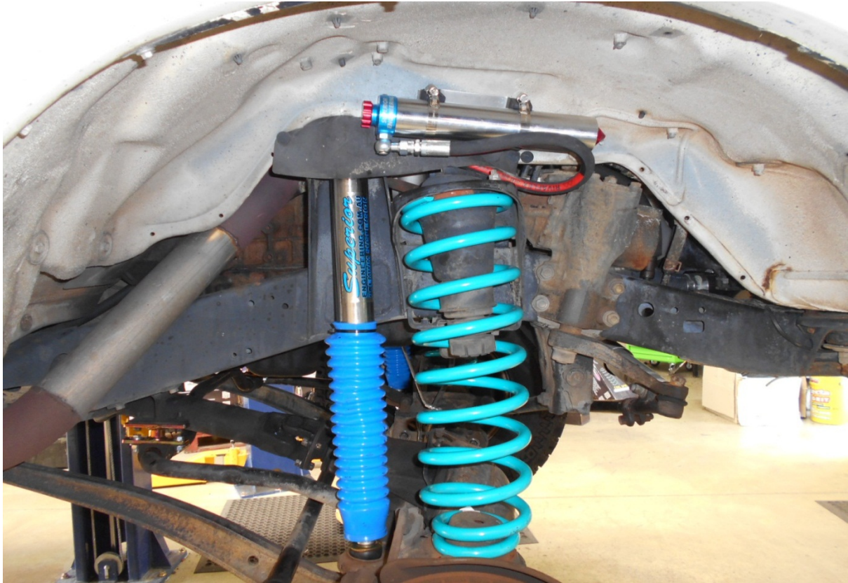
Figure 2: Correctly Fitted Pin Style Shock.
