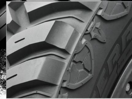
Wide and deep tread pattern features an open shoulder design to further enhance handling, grip, stability and ride quality, while easily expelling mud at high and low speeds
