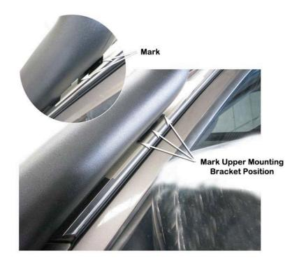
Remove the snorkel body (item 1) from the vehicle and remove the upper mounting bracket (item 3) from the snorkel body.
