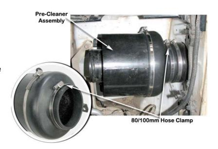
Align the two hoses (items 10 &12) for best fitment, ensure that the snorkel outlet hose (item 10) is installed hard up against the shoulder of the snorkel body outlet snout, tighten the 100/120mm hose clamp (item 15).
