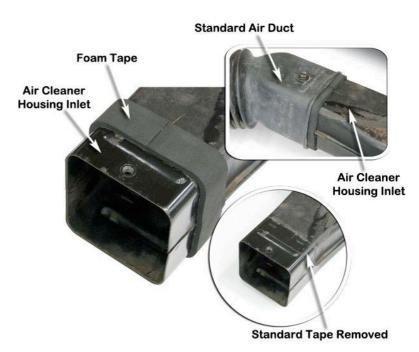
Apply sealant to the inside of the standard air duct and to the outside surface of the pre-cleaner housing outlet, install the standard air duct onto the pre-cleaner housing outlet, secure with the standard hose clamp.
