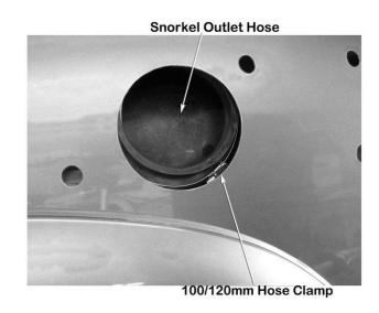
Carefully install the snorkel body (item 1) to the guard panel guiding the snorkel body outlet snout into the snorkel outlet hose (item 10), align the snorkel body to the guard panel and upper mounting bracket.
