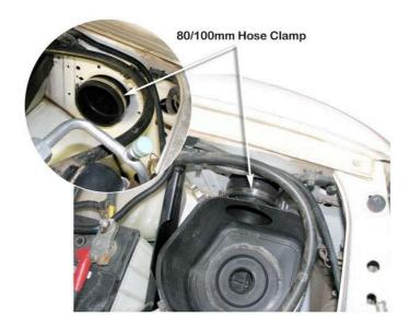
Align the two hoses (items 10 &12) for best fitment, ensure that the snorkel outlet hose (item 10) is installed hard up against the shoulder of the snorkel body outlet snout, tighten the 100/120mm hose clamp (item 15).
