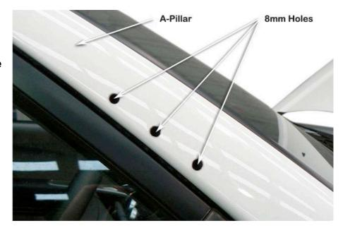
Secure the upper mounting bracket (Item 3) to the A-Pillar using 3 x self tapping screws (Item 5)
