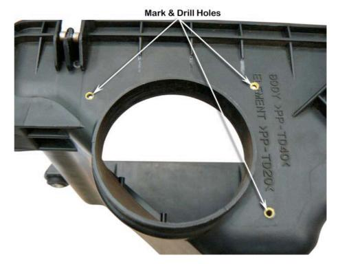
Apply a liberal amount of adhesive sealant to the air cleaner adaptor flange (Item 12) and around the external surface of the air cleaner inlet snout.
