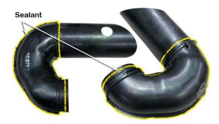
Install the lower air transfer duct into the air cleaner base.
