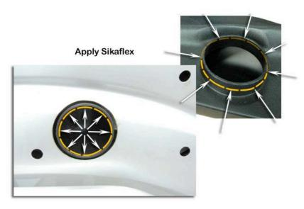
With the snorkel body correctly positioned, fasten to the guard using a body washer (Item 8) and Nyloc nut (Item 9) on each of the stainless steel mounting studs previously installed into the inserts in the snorkel body.
