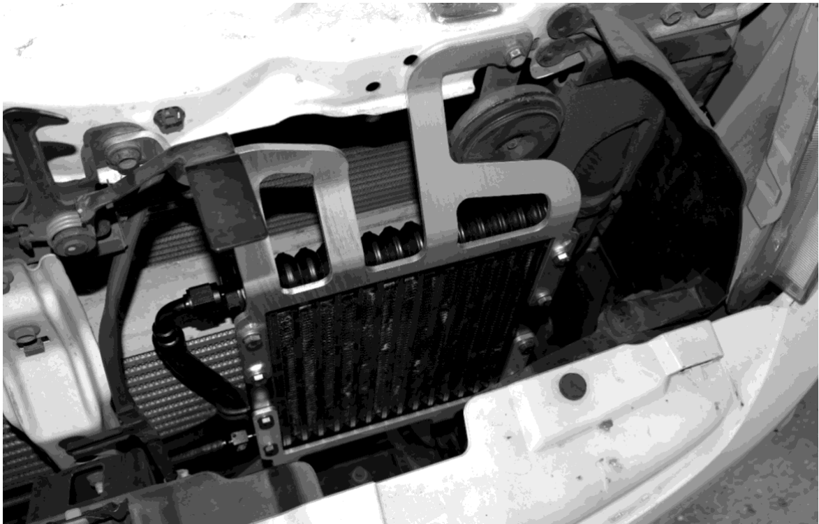
Transmission Cooler Assembly Bolted in Place.
