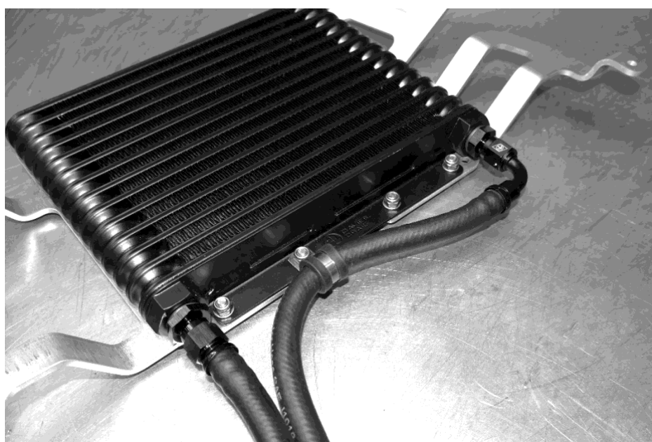
Image shows P-clip mount location and hose path, viewed from behind before being installed (to show detail)
