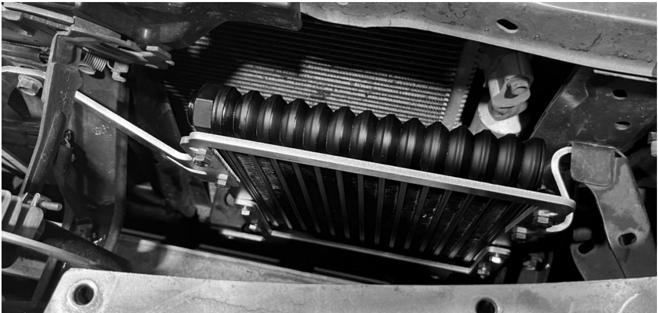
Transmission Cooler Assembly Bolted in Place. Note: Fittings not shown in image.
