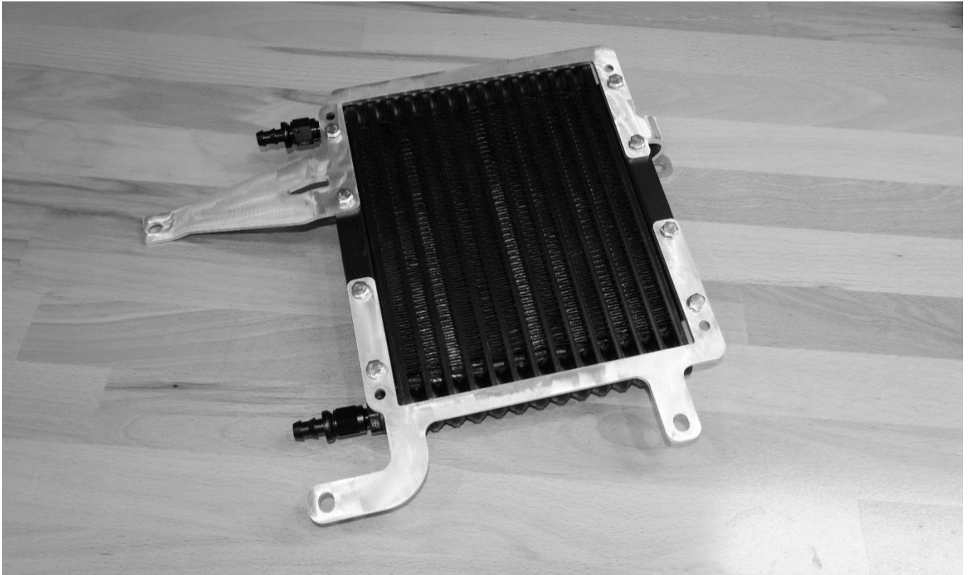
Cooler assembly with fittings in place at correct orientation
