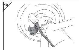
At the point the wiring enters the cabin, ensure there is a loop of cable below the level of the entry point to reduce risk of water ingress.
