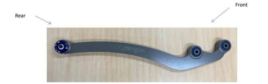
• Note for 2016 and onwards models for 70 series vechiles, there will be a left and right hand version due to arm curvature
