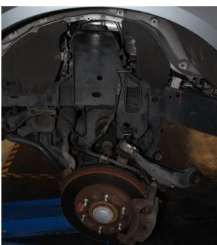
Picture 1: Front Strut Removal
