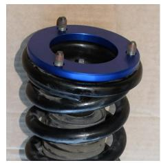
Picture 2: Strut Spacer on Strut
