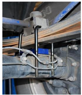
Picture 3: Installation of Raising Block
