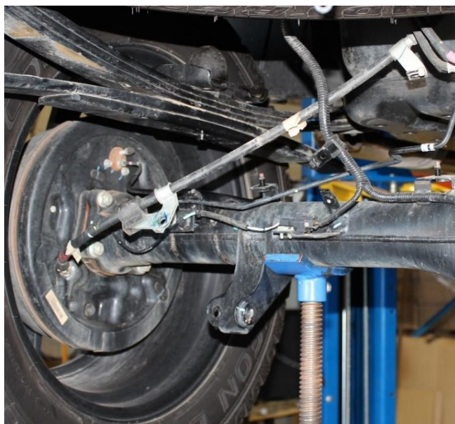
Picture 2: Raising Block Installation
