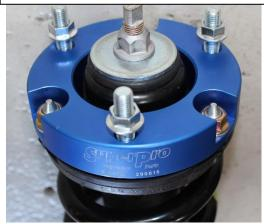
Picture 1: Picture of strut spacer on strut
