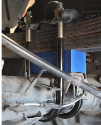
Picture 4: U-bolt and fish plate installation
