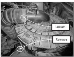
Figure 7– Air intake clamp and lower mounting bolt
