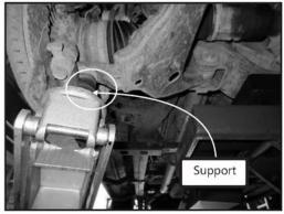
Figure 2- Recommended Lower Control Arm Support
