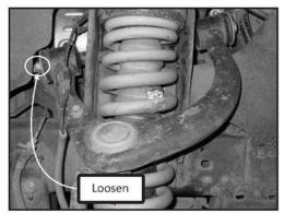
Figure 5 – Control arm bolt loosening.
