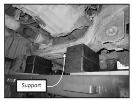
Figure 1- Recommended Chassis Support
