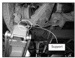
Figure 2- Recommended Lower Control Arm Support
