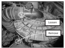
Figure 7– Air intake clamp and lower mounting bolt
