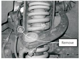
Figure 3 – Removal location of ABS wiring and split pin.
