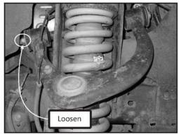
Figure 5 – Control arm bolt loosening.
