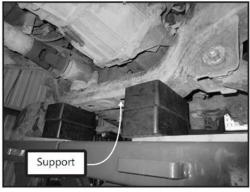
Figure 1- Recommended Chassis Support
