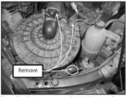
Figure 6 – Air mass sensor and wiring harness clip
