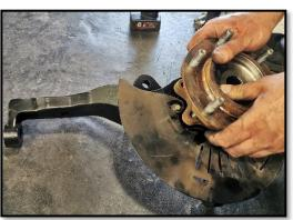
Figure 6: Remove wheel bearing hub assembly & dust shield
