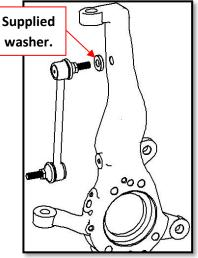
Figure 8: Supplied washer arrangement
