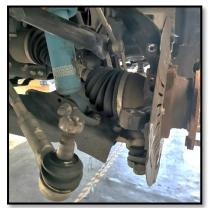
Figure 3: Remove Tie Rod Outer Joint
