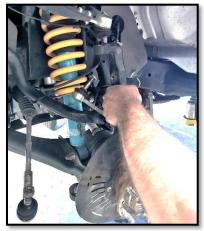
Figure 5: Remove OE steering knuckle from the vehicle
