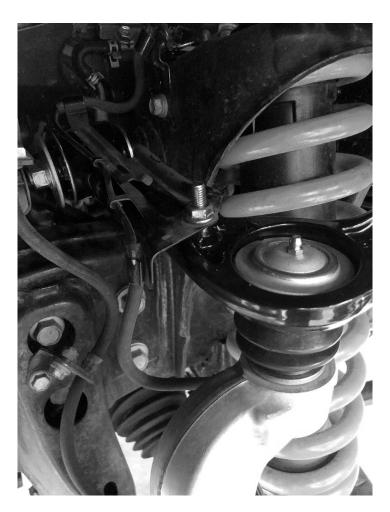
15. Reinstall the headlight sensor bracket to the new arm if fitted.
