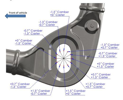
In conjunction with rotating the ball joint, the ball joint can slide in and out in the slot, which allows for +/- 1 degrees of additional camber adjustment.
