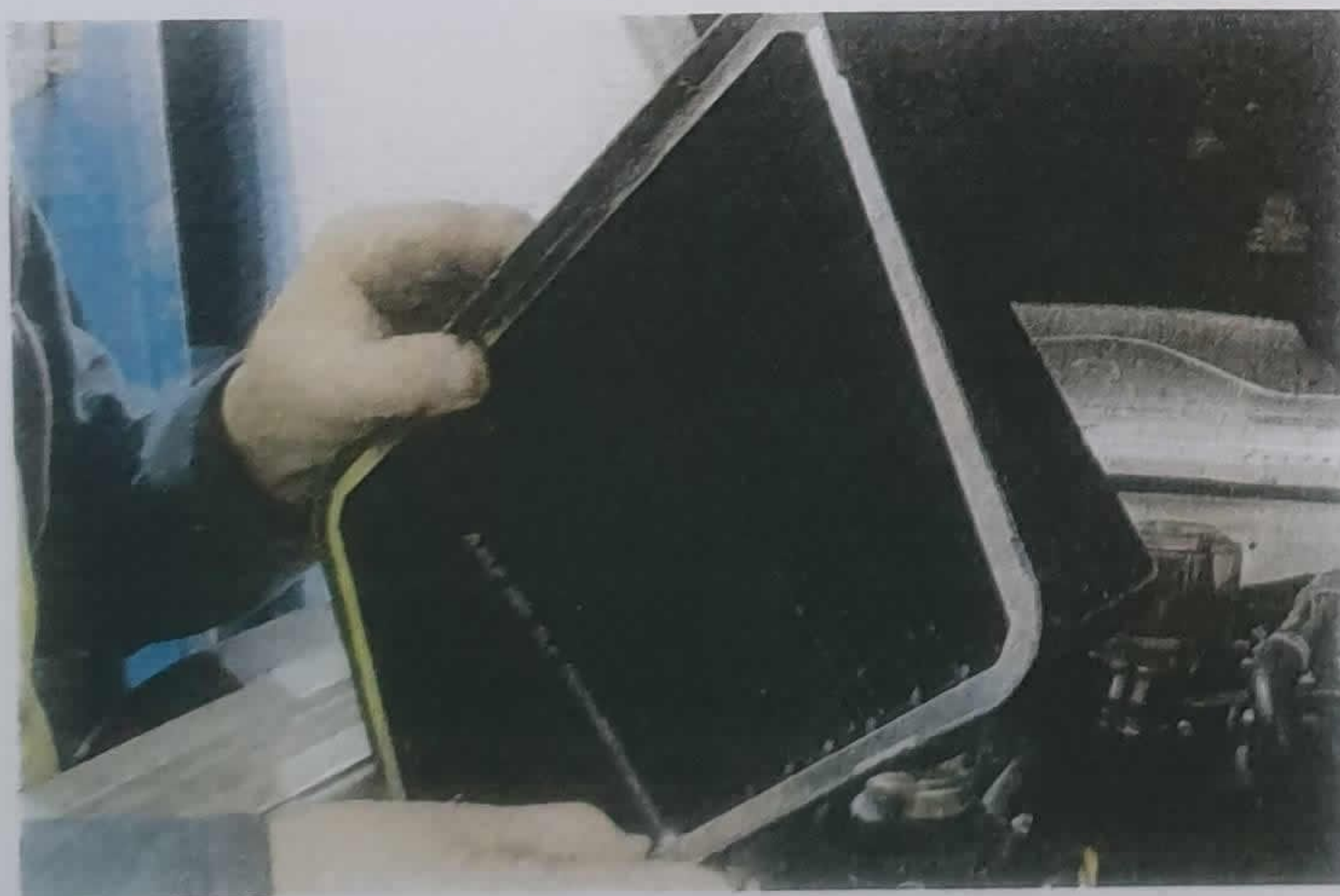
Step 3: Apply sealant to entire surface of one side of insert and bond to upper cover to create an air tight seal.
